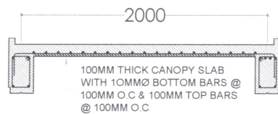
CANOPY DETAILS SCALE: 1:30MM
