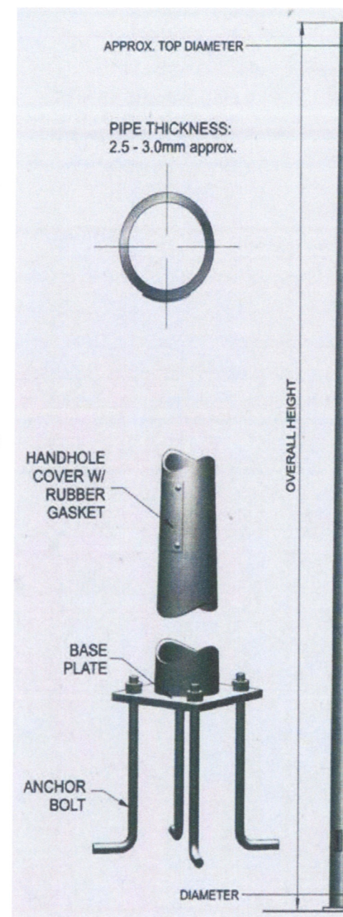
POLE CONNECTION DETAILS
